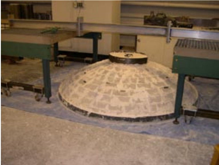
The 7 foot diameter AAC dome ready for testing to failure in the structural lab at MIT
