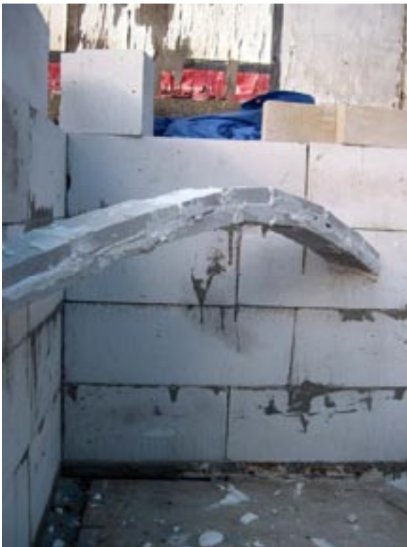
A 4" wide and 2" thick arch of AAC spanning 48" will support over 200 pounds
