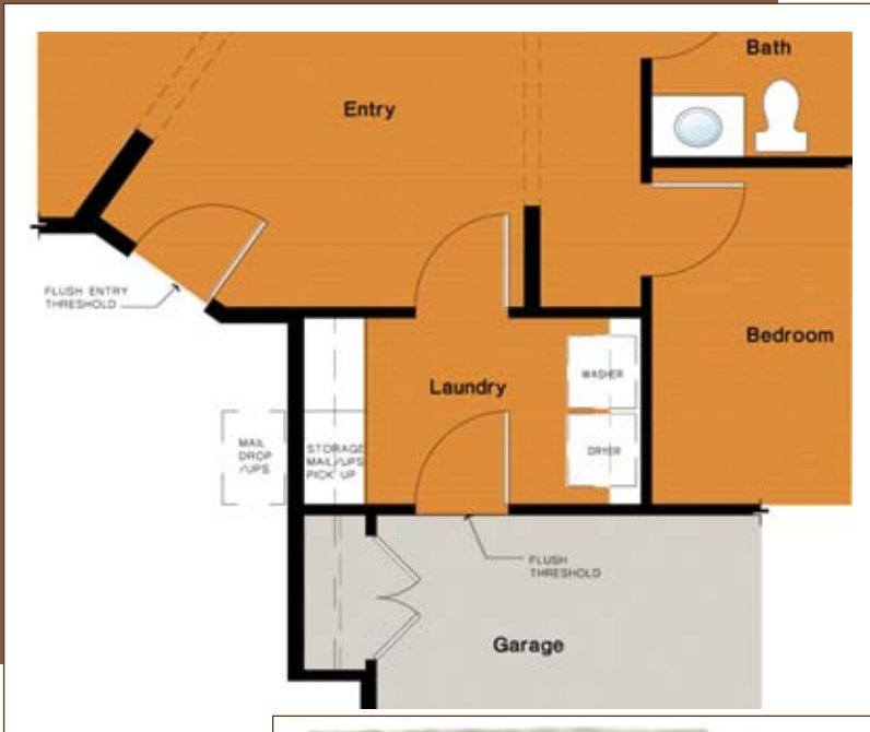
Figure 10a: Floor plan showing location of mail drop/pick-up drawer accessible from laundry room.
