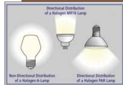
(Figure 5) Different distributions of an A-lamp, a PAR lamp, and an MR 16 lamp
