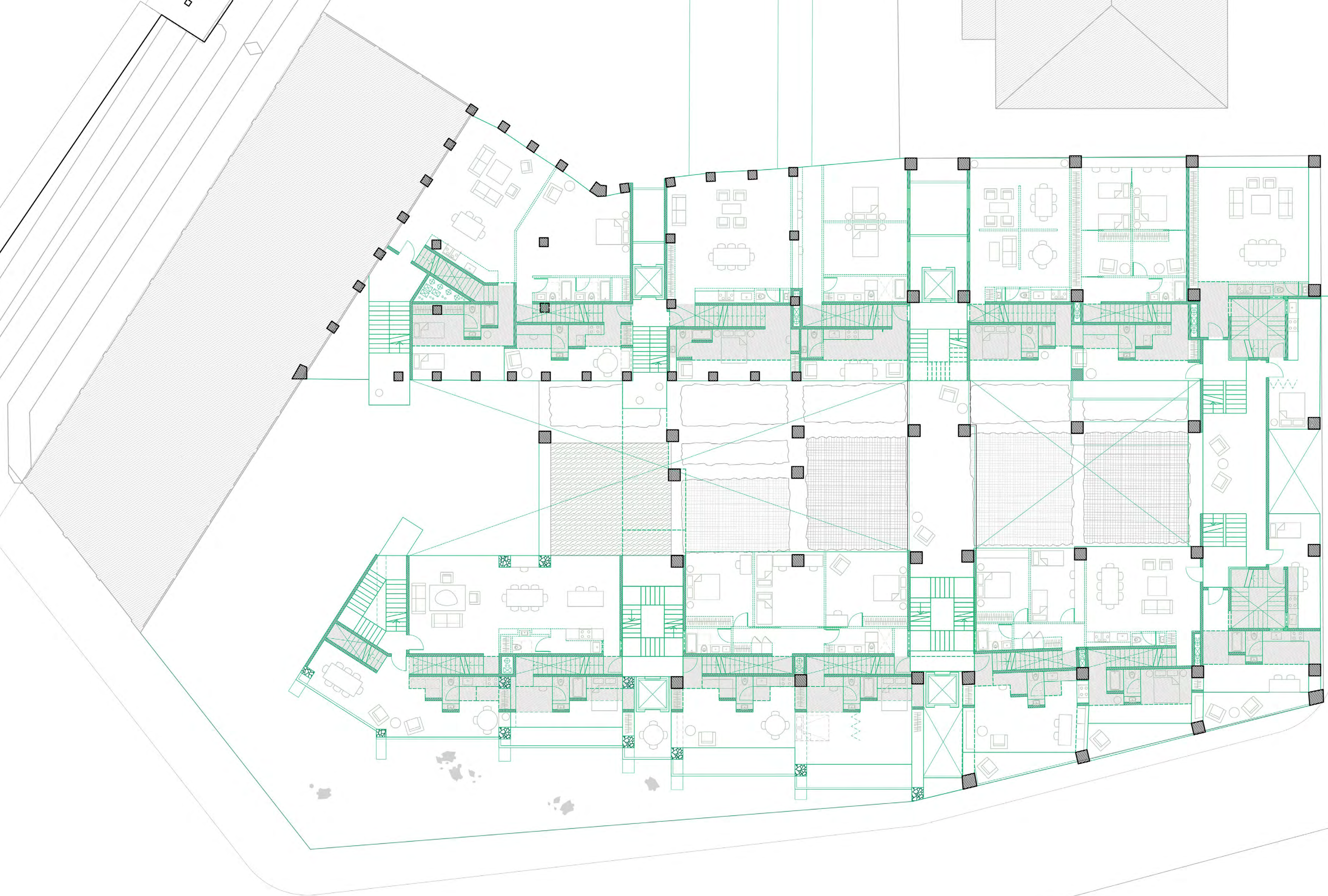
TYPICAL UPPER FLOOR PLAN (Original Structure in Black, Proposed Layer in Teal)
